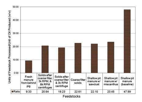
Fig. 2 Relative energy costs per unit of oil production
