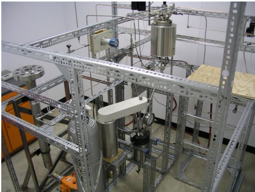
Figure 5. Photo of the CHTP reactor system setup.
